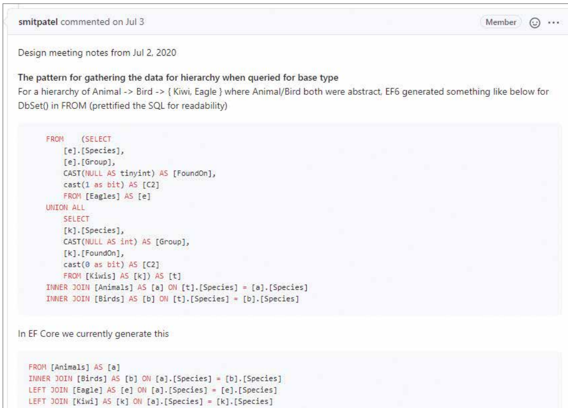
Figure 4: Comparison of SQL generated from a TPT query in EF6 vs. EF Core 5
